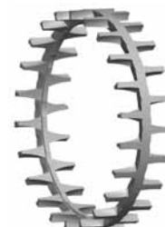
Fig. 6. EMB/YMB One-piece, machined-brass, land-riding, finger-type cage.
