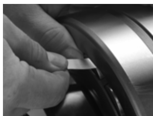
Fig. 14. Measure RIC before installation.
