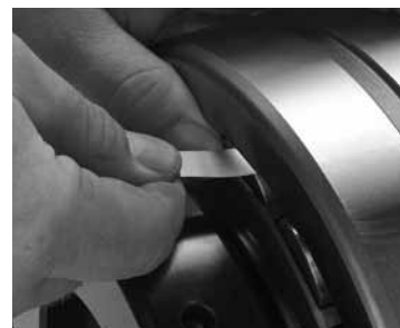
Fig. 18. Measure RIC before installation.
