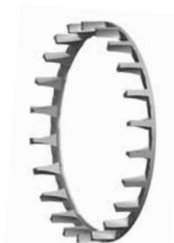
Fig. 7. YMD Split, machined-brass, land-riding, finger-type cage.
